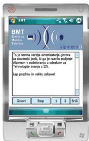
Figure 3: Prototype speech synthesiser developed in the project "BMT: development of a text speech reader for mobile telephones for blind and partially sighted users".
